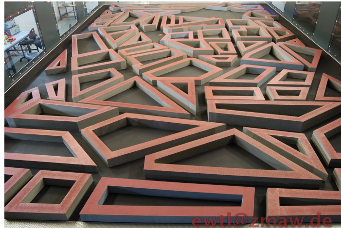
Figure 1: Geometry of the test case "Michel-Stadt" inside the "WOTAN" wind tunnel of EWTL of the University of Hamburg. Flow direction downwards. Figure from (EWTL 2022).
